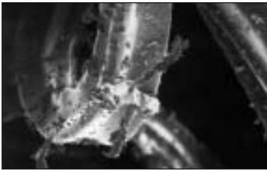
← AFTER SOILING PHOTOGRAPH of the most heavily soiled Sample #1 clearly shows the effects of the sticky detergent residue left on the fibers that attracted and held large and small soil particles. Because the detergent left a heavy sticky residue, soil particles attached themselves quickly and tenaciously to the fibers and caused the carpet to resoil more rapidly.
