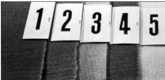
Number One was cleaned with a steam machine (hot water extraction and detergent); Number Two with a rotary brush machine; Number Three with a dry-foam machine with built-in vacuum to remove soil; Number Four with a reel-type machine without vacuum pick-up and stock detergent. Sample Number Five served as the control piece and was not cleaned or exposed to foot traffic or soiling.
